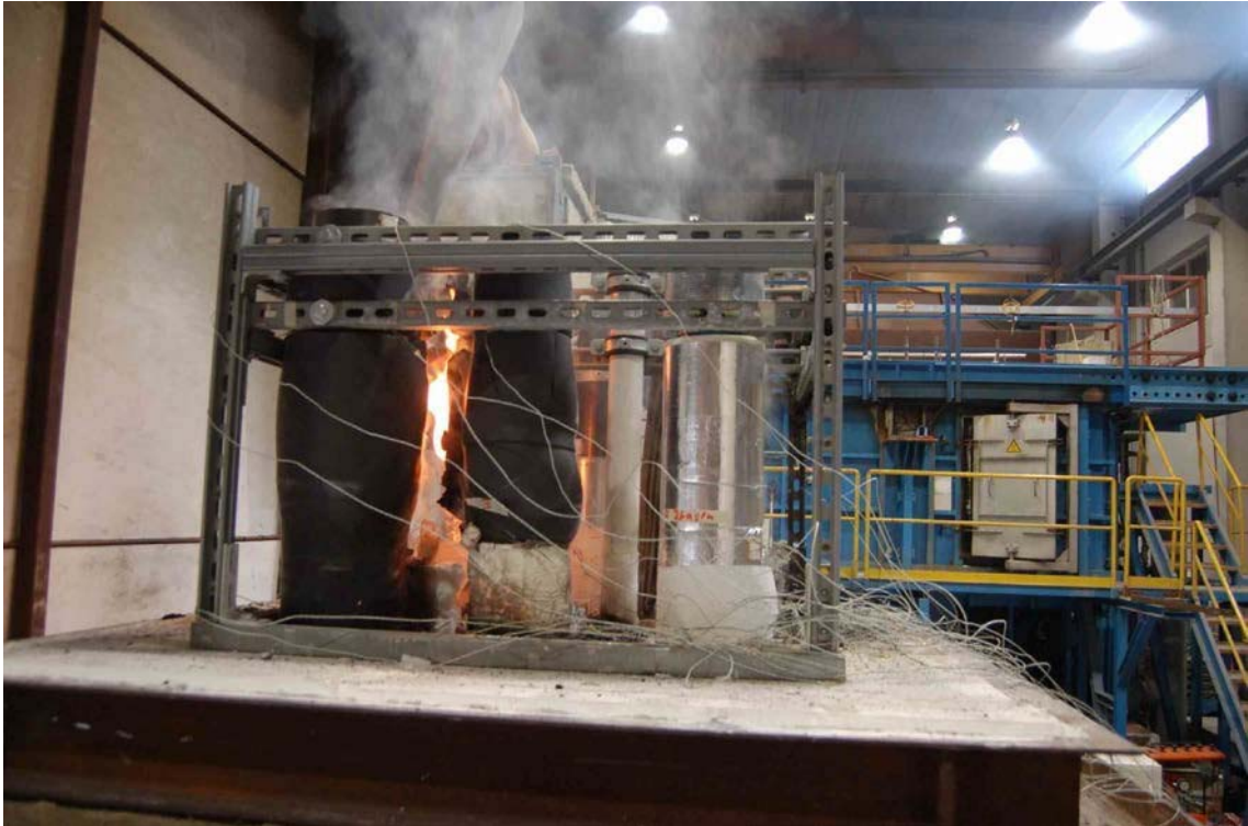
Photograph 11 Specimens after 152 minutes of heating (end of heating after consulting the client)
