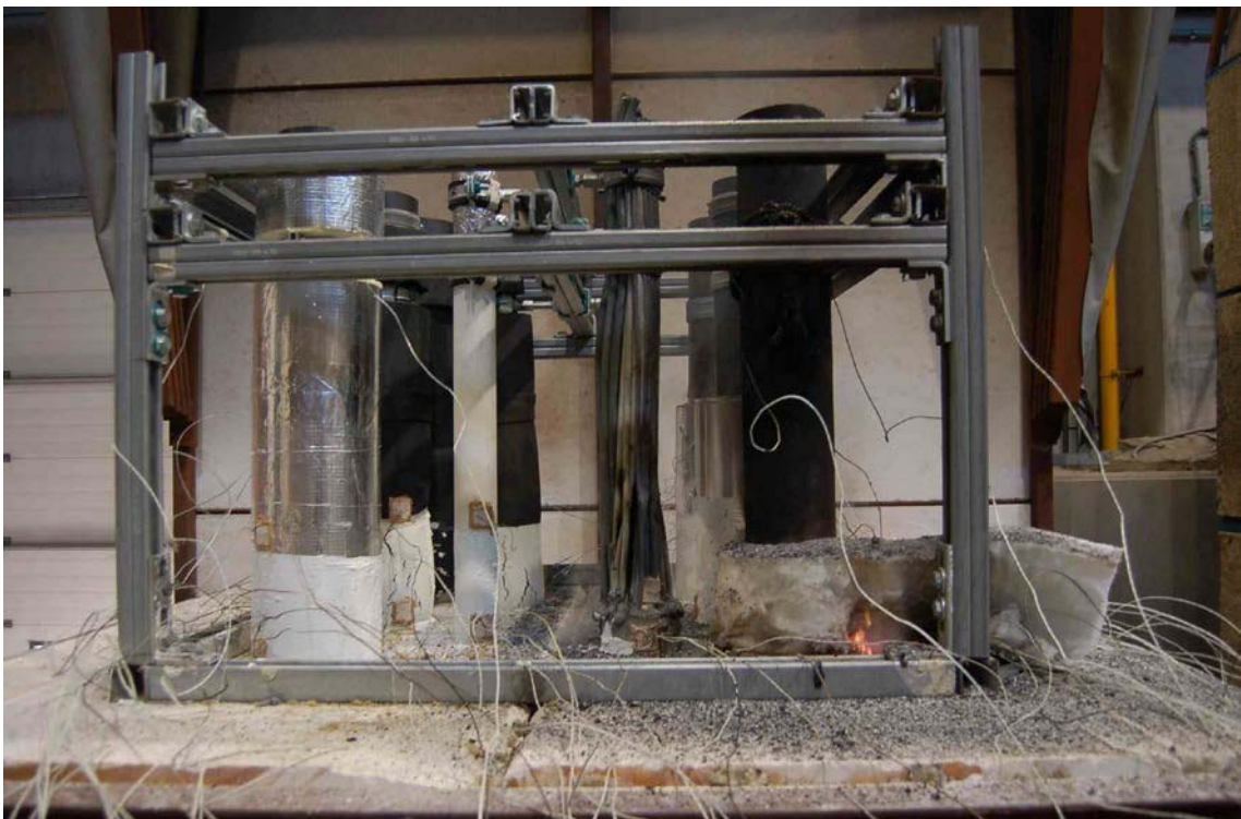
Photograph 6 Specimens after 28 min of heating
