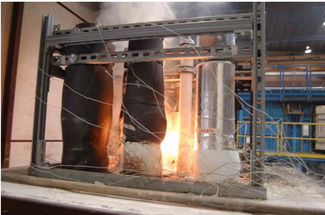
Photograph 10 Specimens after 101 min of heating, flaming on service no. 8
