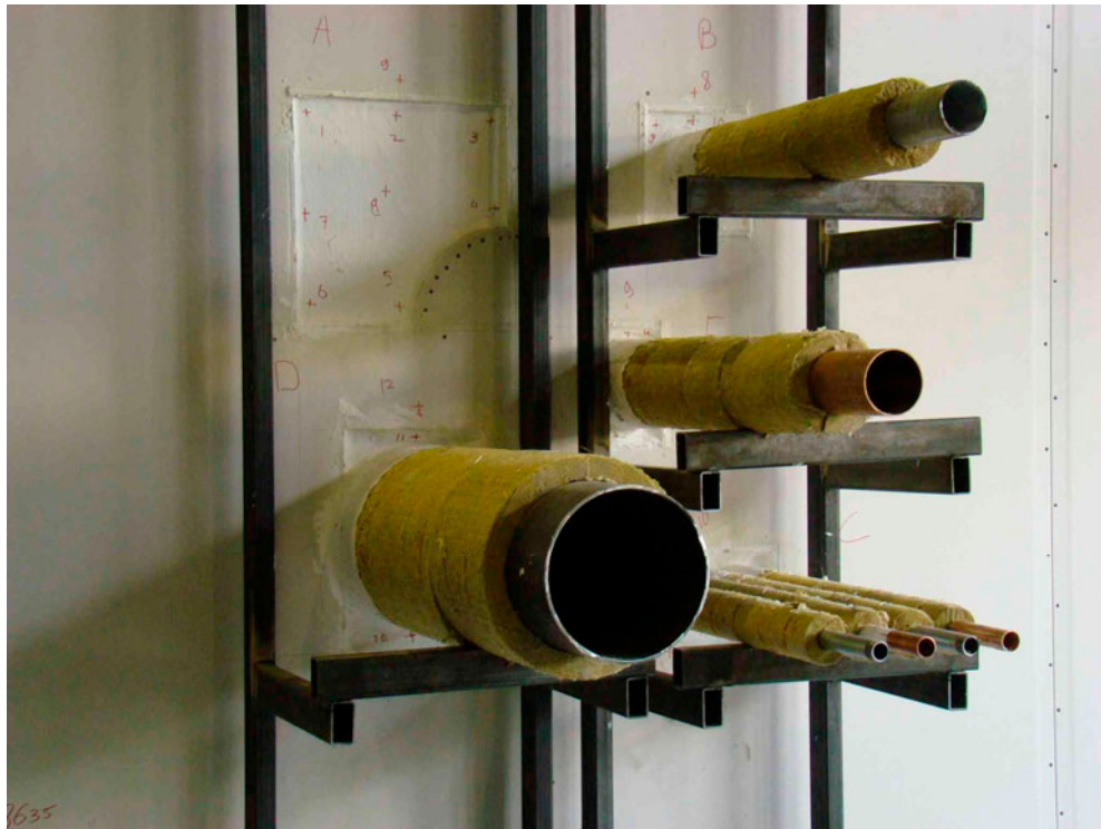
Photograph B1 Specimen before the fire test seen from the non exposed side
