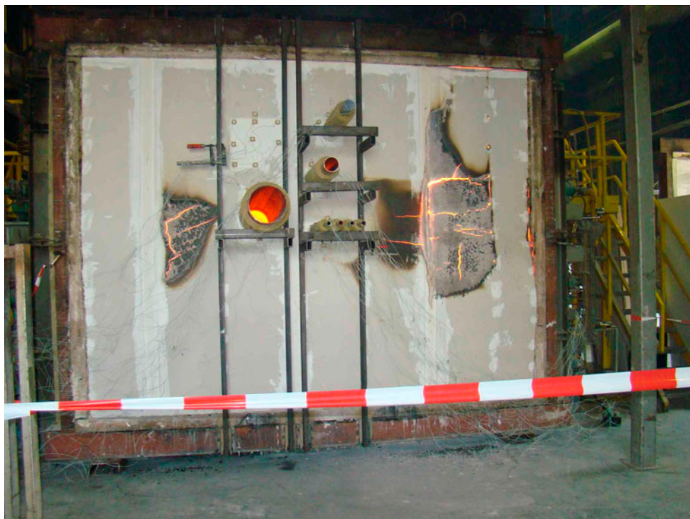
Photograph B2 Specimen seen from the non exposed after 76 minutes of heating
