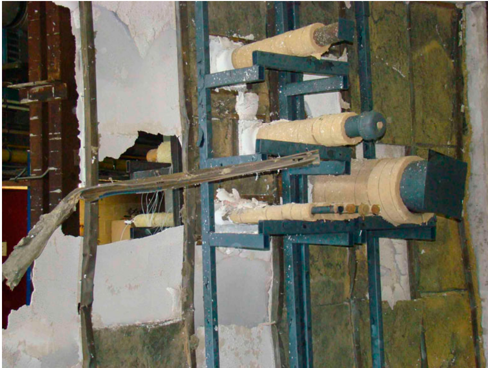
Photograph B3 Specimen after the fire test seen from the direct exposed side
