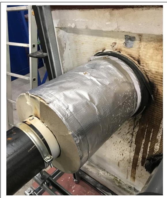
Pipe No. 5 (steel pipe, InsulPIR) Variant N III wrap, C/U
