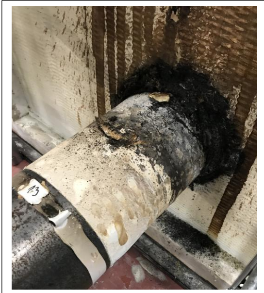
Pipe No. 1 (steel pipe, 300mm Flamro BMA) Flamro DSB-W Kit, C/U
