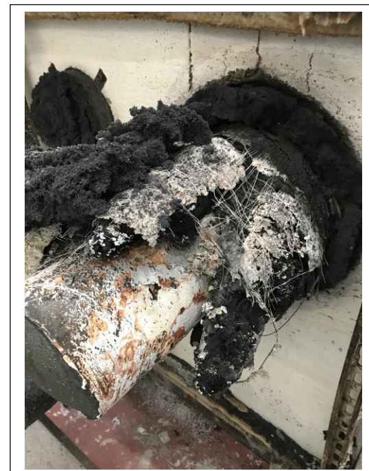
Pipe No. 5 (steel pipe, InsulPIR) Variant N III wrap, C/U
